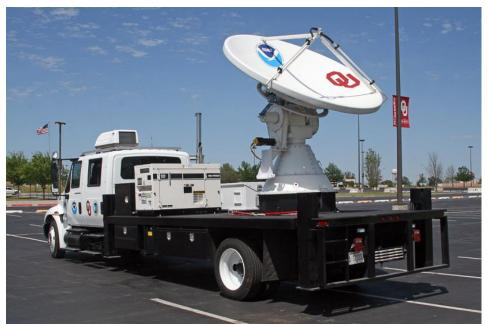
The NOXP mobile radar can be driven into position as a storm is developing to rapidly scan the atmosphere at low levels, below the beam of WSR-88D radars. CIMMS and NSSL researchers use mobile radars to study tornadoes, hurricanes, dust storms, winter storms, mountain rainfall, and even swarms of bats.
