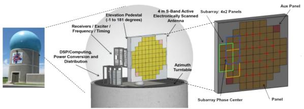
The ATD is a proof-of-concept system to demonstrate improved capabilities and refine the cost-driving requirements of a multifunction phased array radar (MPAR). It is an S-band, mid-scale, dual-polarized, multifunction, active, electronically scanned PAR at the National Weather Radar Testbed (NWRT) in Norman, OK.
